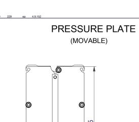
Space between pressure plate and supporting column should be kept free from fixed installations!
